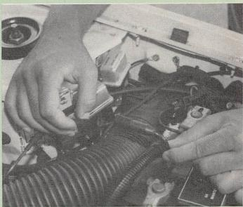
Modern cars use connectors for just about every current path. So if you want to disconnect some equipment when taking current readings, it might be easier simply to open the appropriate battery connector than to start disconnecting wires at the particular device you want to disable.
