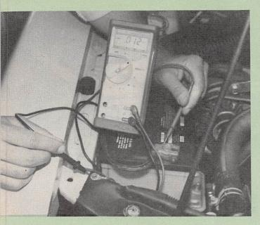
measurement tells you if a thermostat—such as the one that controls a fan—is working properly.
