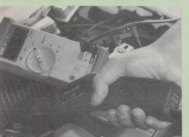
Having electrical problems with lights, fans, etc.? Often the problem is a high resistance between the battery's negative terminal, and the chassis and engine block. Don't make resistance tests; they are worthless in this instance. Instead, turn on the maximum current load and measure the voltage drop between the battery's negative terminal and the chassis/body. It should be well under 1 volt—usually in the millivolts range.
