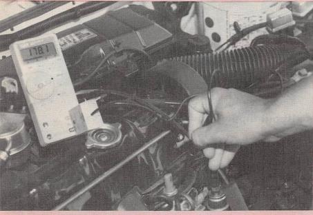
Having heat problems with the engine, the radiator, the heater? You can track them down with a thermistor temperature probe (a device that converts temperature to a DC voltage that can be read on a DC voltmeter in terms of temperature). Here the probe shows that the engine temperature is too low, possibly indicating that a thermostat is stuck open.
