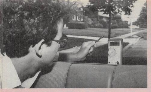
The individual wires in the rear window defogger can be tested by connecting one probe of a voltmeter to the power connector on one side of the defogger and then sliding the other along each "ceramic wire." The voltage reading will decrease as the probe is moved along the wire. If the reading suddenly drops out, the probe has passed over a break in the "wire."
